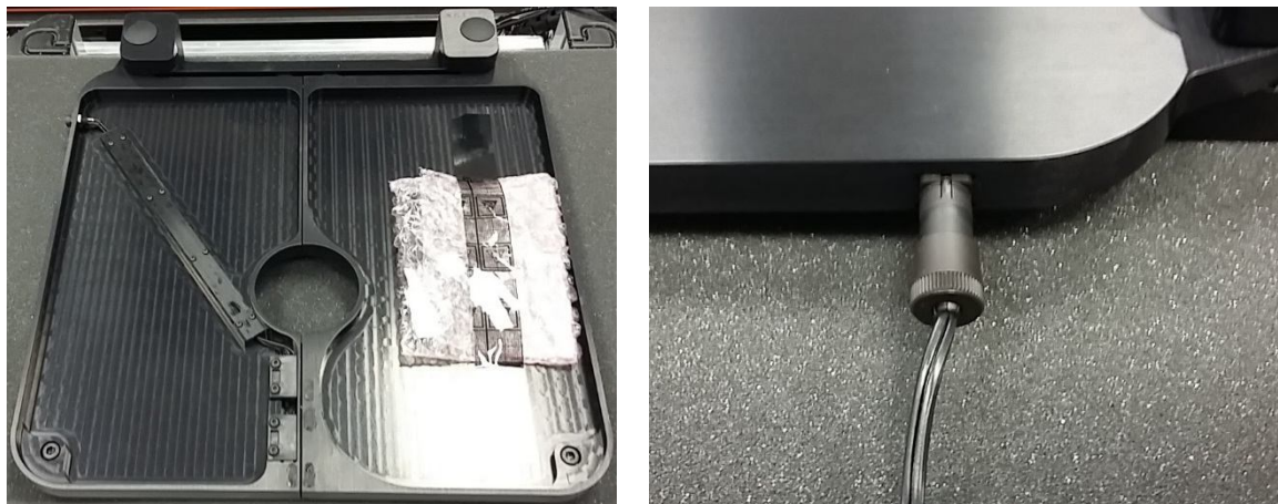
Figure 5: External Interlock Cable (ASE-11399) in Bag Underneath Stage Cover and Connected
